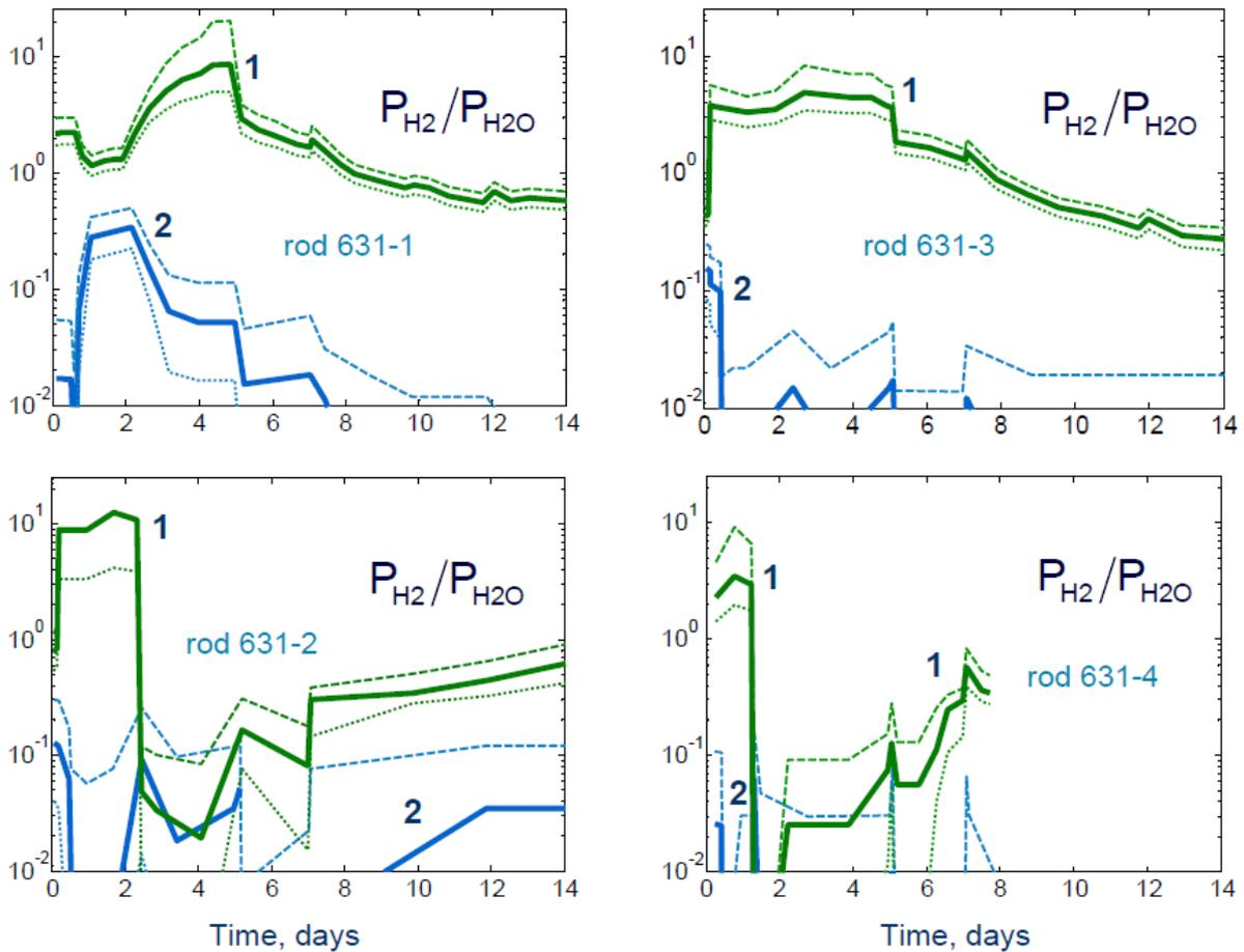
Fig.7. Evolution of hydrogen-to-steam ratio after simulation of the primary failure – as inferred from the data [3]. Lines in green color (1) are for the lower part of the rodlets with higher heat rate (area of secondary hydriding), lines in blue (2) are for the upper part of the rodlets (the low temperature domain). Dashed lines show the uncertainty boundaries for solution of the inverse problem.
