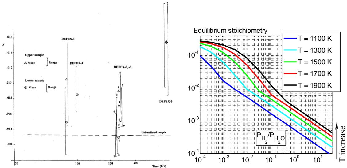
Fig.9. *a* – The DEFEX PIE data on fuel stoichiometry, [4]. *b* – Equilibrium deviation ( $x$ ) from the stoichiometric composition of  $UO_{2+x}$  at different temperatures as a function of hydrogen-to-steam ratio in the gas phase.
