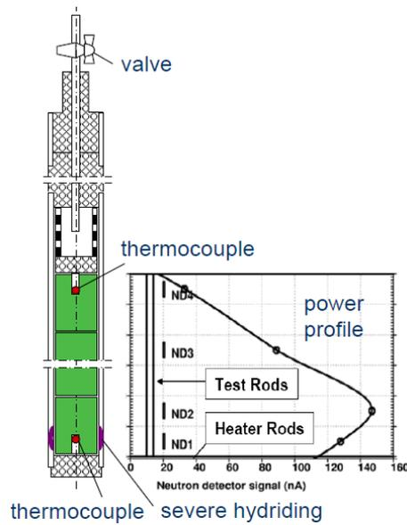
Fig.3. The scheme of the IFA-631 test rodlets and the axial power profile during irradiation.
