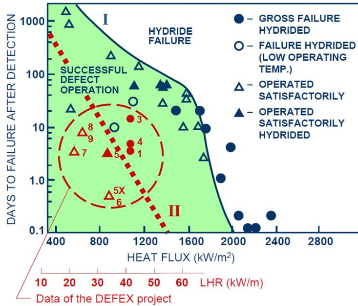
Fig.1. The Locke diagram. Dark-blue markers and line I are the experimental data and the Locke criterion of secondary failure, respectively, [2]. Green area is the range of parameters for successful operation of fuel rods with a primary defect. Red markers are the data of the DEFEX project, [4] (the corresponding linear heat rates are shown below in red color); line II is the rough boundary separating the DEFEX tests with successful fuel operation from that with secondary failures.
