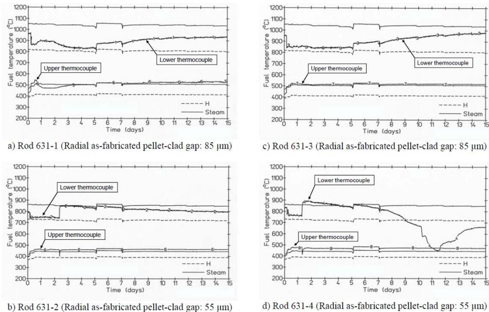
Fig.5. Thick lines – TC readings in the test rodlets during the first 15 days after simulation of the primary failure. Thin lines – centerline temperature calculated for the TC axial positions with the FTEMP code under the assumption that the gas in the pellet-to-cladding gap is pure hydrogen (dashed line) or pure steam (solid line). Reproduced from [3].
