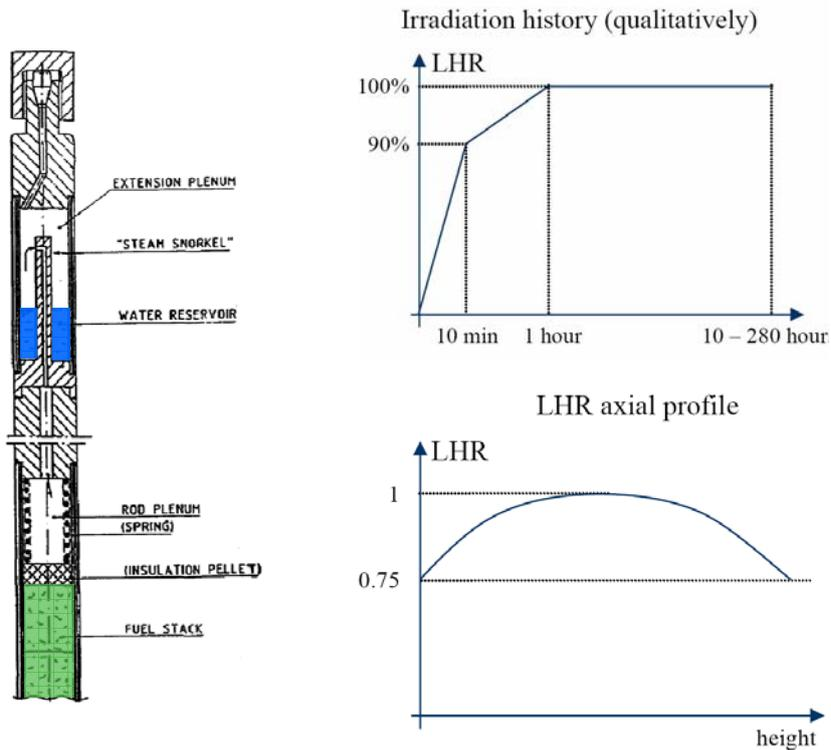
Fig.8. Data to the DEFEX project, [4]: *a* – a scheme of the test rodlets; *b, c* – sketches for linear heat rate history and axial power profile, respectively.
