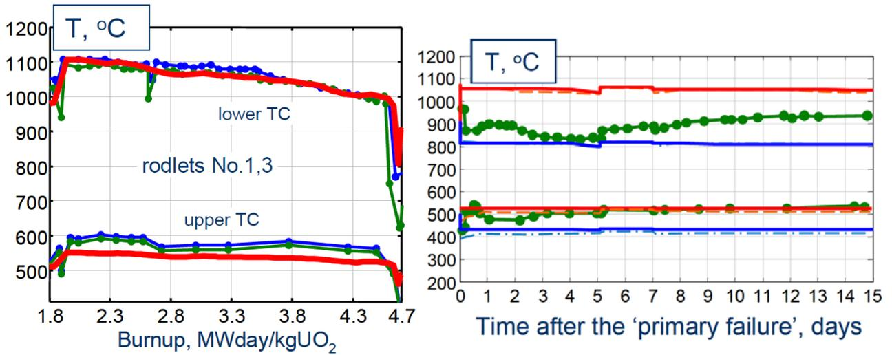
Fig.6. The RTOP-CA calculations for rodlet 631-1 compared to the TC data.
