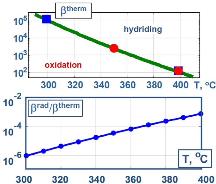
Fig.2. *a* – The out-of-pile data on the threshold of massive hydriding: ● – sponge Zr at total gas pressure of 70 atm [5], ■ – Zircaloy-2, 1 atm [7]. *b* – The change of the threshold under irradiation as estimated in Ref.[8].
