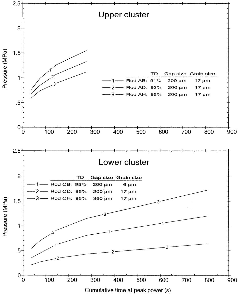
**Figure 9. Fission gas released for the fast ramped IFA-535.5 and the slow ramped IFA-535.6 rod as a function of time**
